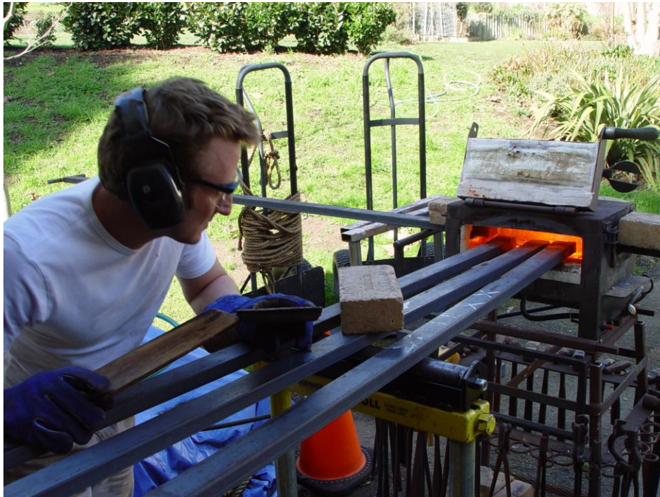
The thick bridge and fence posts are hand-forged Cor-ten steel. The artists use traditional blacksmithing techniques to individually shape each one of the posts. Artist David Duskin monitors the steel posts in the forge as they heat to a malleable temperature.
